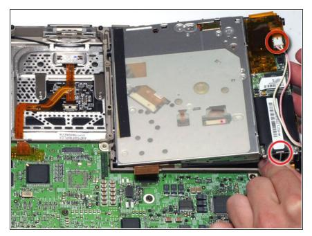
Lift the drive up on the right side so that you can access and disconnect the modem cable and inverter cable.
