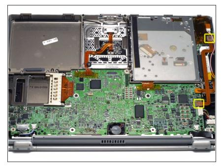
Disconnect and remove the indicated orange ribbon cable.
