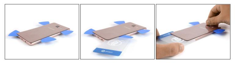
Insert a plastic card at the bottom and slide it underneath the back cover.
