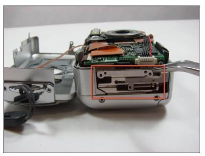
• Use a pair of <u>tweezers</u> and remove the metal piece inside the camera.
