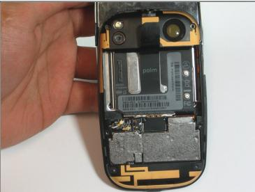
• Use the t4 screwdriver to remove all 6 of the 3.6mm long screws.
