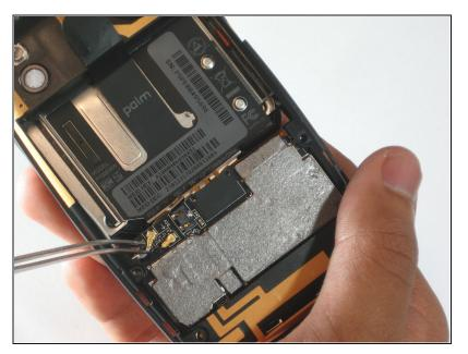
Use <u>tweezers</u> to remove the DIV and GPS antennas from the back of the keyboard.
