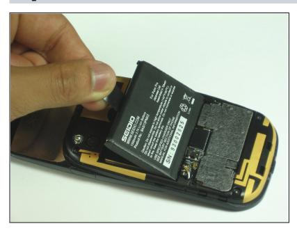
Carefully pull up on the tab to remove the current battery.
