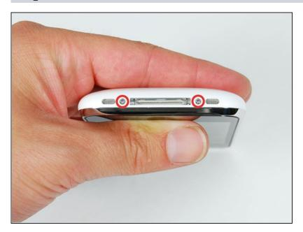
• Remove the 2 Phillips #00 screws at the bottom of the iPhone, located on both sides of the dock connector.
