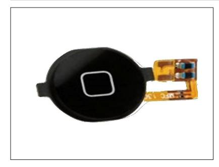
If any cables or pins are broken , you could buy new cables, as mentioned before. However, if the home-button screws are broken or missing, or the home-button is completely broken, you might want to buy a new home button assembly. This assembly is displayed on this step's adjoining image.
