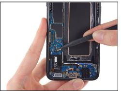
• Use the point of a spudger to disconnect two antenna cables that connect the motherboard to the daughterboard.
