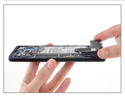
Remove the loudspeaker assembly.
