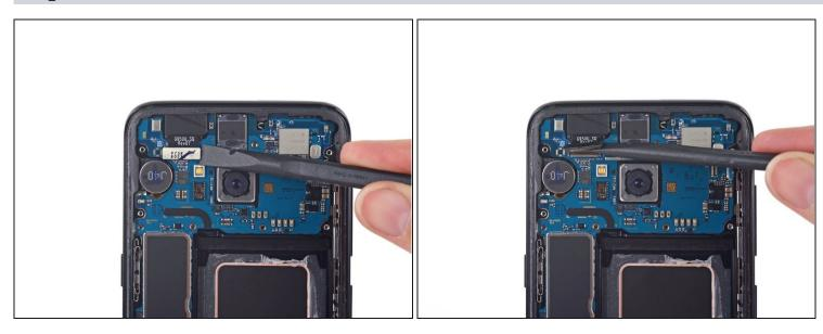
• Use the flat end of a spudger to disconnect the front-facing camera connector.
