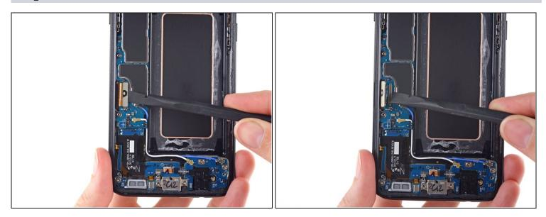
• Use the flat end of a spudger to disconnect the display and digitizer connector.
