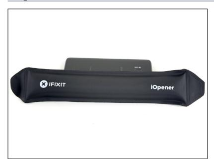
Once you have the tool firmly inserted into the glass, reheat and reapply the iOpener to soften the adhesive.
