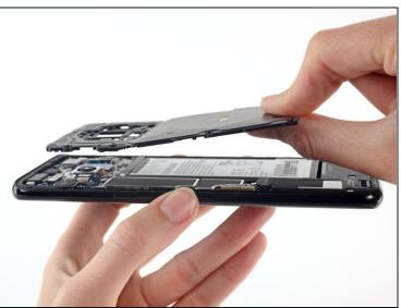
• Remove the NFC antenna and charging coil assembly.
