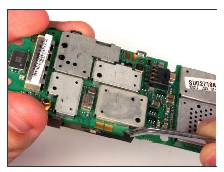
Use tweezers to pry off the four clasps that hold the display in place.
