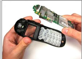
Remove the motherboard by lifting it up and out.
