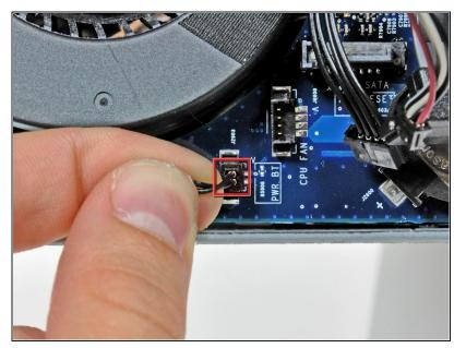
Pull the power button cable connector up off its socket on the logic board.
