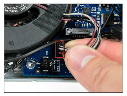
Disconnect the CPU fan by pulling its connector up off the logic board.
