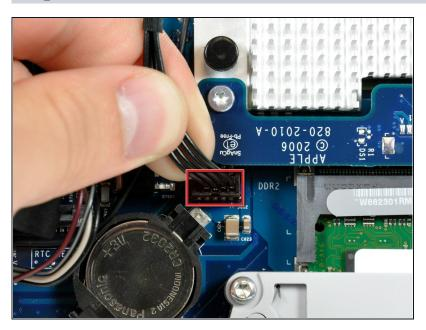
Disconnect the hard drive power cable by pulling its connector up off the logic board.
