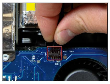
• Disconnect the optical drive thermal sensor cable from its socket on the logic board.
