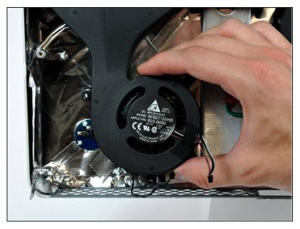
• Lift the CPU fan out of the rear case.
