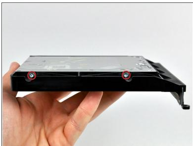
Remove the two 6.5 mm T10 Torx screws from both sides of the optical drive (four screws total).
