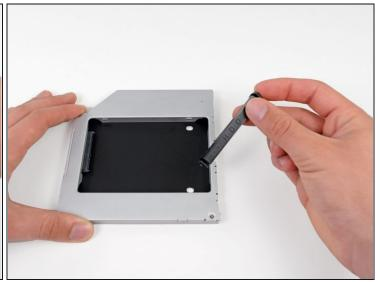
• Remove the plastic positioner from the optical bay hard drive enclosure by pressing in on one of the clips on either side and lifting it up and out of the enclosure.
