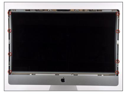
Remove the eight T10 Torx screws securing the LCD to the outer case.
