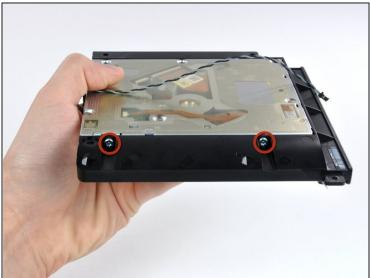
• Remove the two T10 Torx screws from each side of the optical drive (four screws total).
