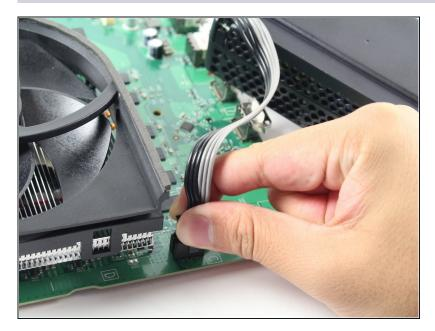
• Grab the connector as shown, pinch the small black locking tab, and pull firmly upward to detach the power block from the motherboard .
