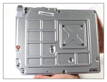
• To remove the optical disc drive, remove the silver 10 mm T-10 Torx screw labeled "C4."
