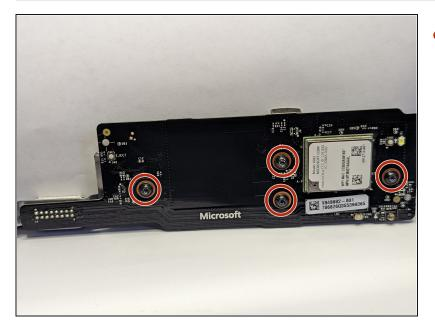
Remove the four black 8 mm T-9 Torx screws labeled "E1," "E2," "E3," and "E4."
