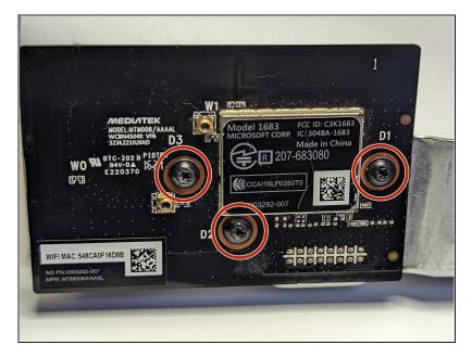
Remove the three black 8 mm T-9 Torx screws labeled "D1," "D2," and "D3" to remove the Mediatek board.
