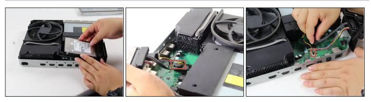
Gently disconnect the hard drive from the motherboard (at the two plastic connector bodies).
