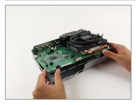
Now that the clamp is removed, gently lift the motherboard from its edges out from the metal casing. The motherboard should come out with ease.
