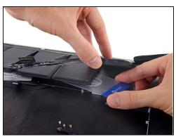
Repeat the above procedure to separate the last remaining battery cell from the MacBook Pro's upper case.
