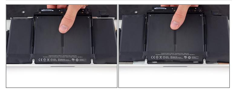
• Lift the battery with the plastic frame and slide it back toward the MacBook Pro's hinge until it clears the screw posts holding it to the upper case.
