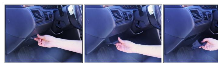
Reach underneath the steering wheel. Then, place your hand to the left to remove the fuse box cover.
