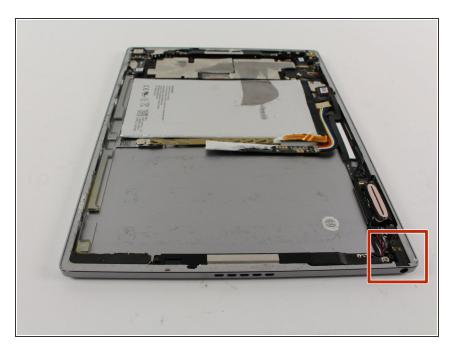
Orient the device so that the headphone jack is in the bottom right corner.
