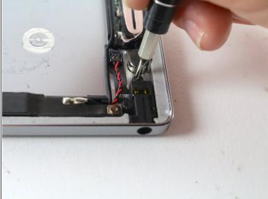
Remove the two 3.5mm Phillips #000 screws.
