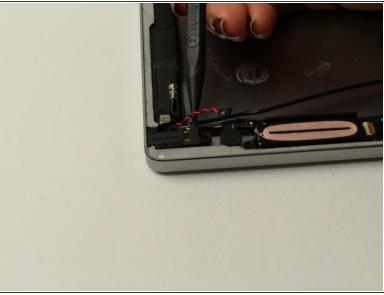
Detach the red and black cable using a narrow spudger.
