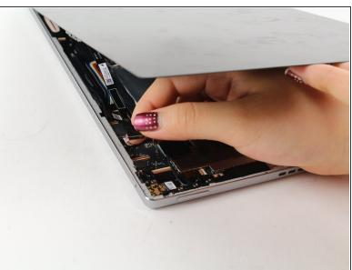
Detach the cables for the camera by lifting the small flap using the tip of your fingernail or a spudger. Gently pull the ribbon cable out.
