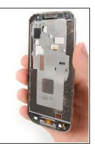
Remove the LCD screen and digitizer assembly completely.
