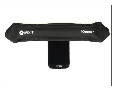
Use a heat gun or an <u>iOpener</u> to soften the adhesive underneath the perimeter of the screen.
