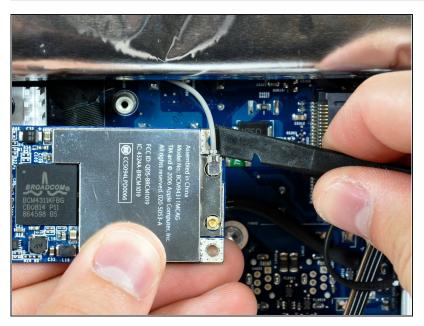
Use a spudger to pry the antenna connector up off the AirPort Extreme card.
