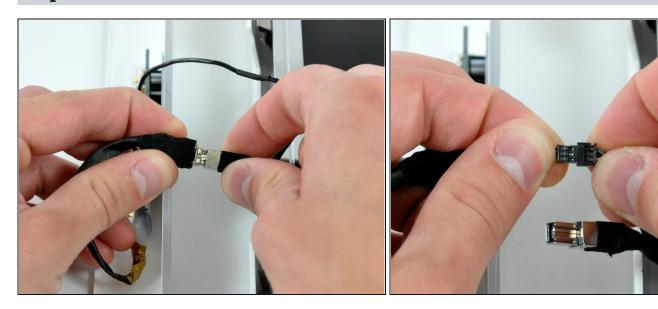
Disconnect both the camera and microphone cables.
