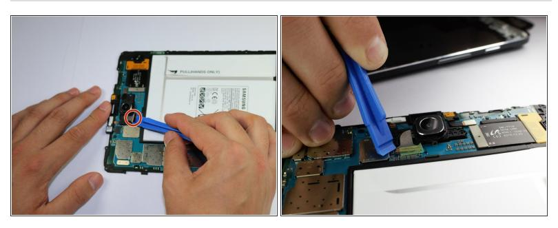
Use the plastic opening tool to detach the camera's ribbon from the motherboard.
