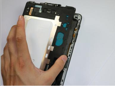
• Use the plastic opening tool to lift and remove the plastic motherboard cover.
