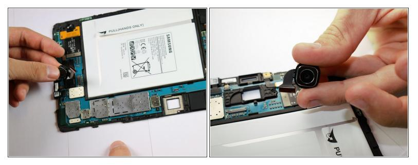
Carefully remove the camera from the motherboard.
