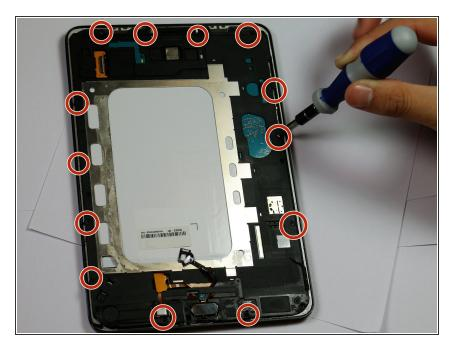
Remove the 13 3mm screws from around the edges of the board using a Phillips #1 screwdriver head.
