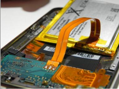
Flip the battery over and place it in the rear panel, face down.
