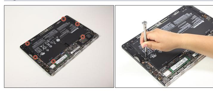
• Remove the six #0 3.8mm Phillips screws from the battery.
