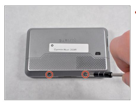
Remove the two 4mm T5 Torx screws.
