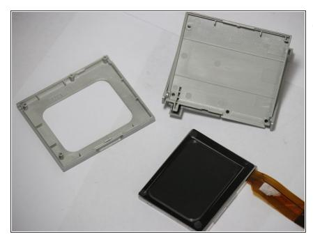
You can now separate the individual pieces from each other, allowing the screen to be accessible to replace.
