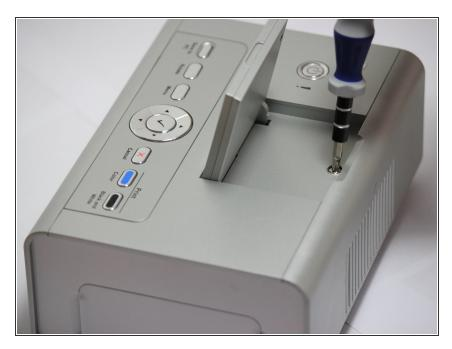
Rotate the device so that it is upright again. Under the LCD Panel there is a 9.62 mm screw, unscrew using a Phillips #2 screwdriver.
