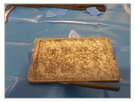
Use Jimmy to Separate screen from back cover. There is a thin gap. use picks to keep gap open while working around all edges.
