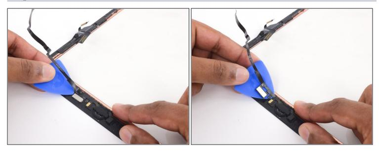
• Insert an opening pick between the metal shield and the front panel and gently pry it from the digitizer.
