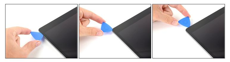
• Rotate the pick around the top-left corner of the device to separate the adhesive.
