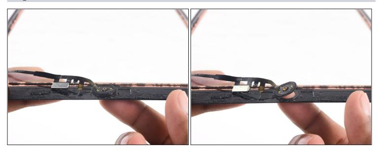
Press the home button from the external side of the digitizer to break up the adhesive holding it in place.
