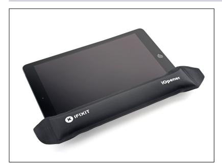
Heat an iOpener and apply it to the left edge of the device for two minutes.
