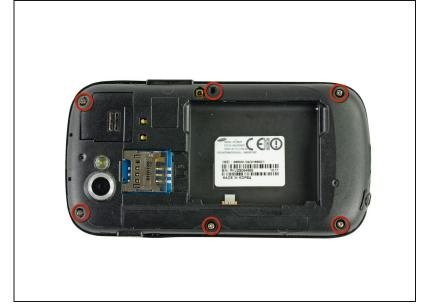
Remove the six Phillips screws securing the rear inner frame to the inner case.
