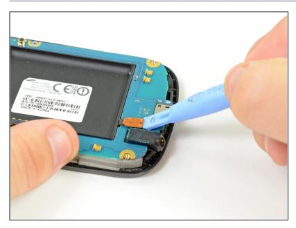
Insert the flat edge of a plastic opening tool underneath the headphone jack connector and pry upwards.
