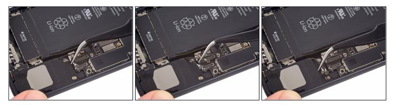
• Use tweezers to gently derout the antenna cables from the metal bracket on the logic board.
