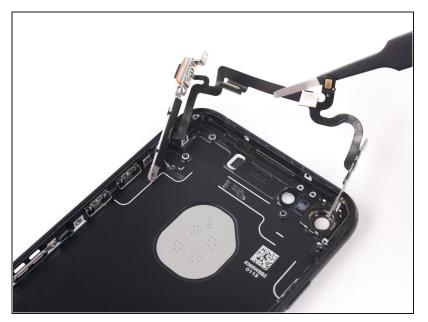
• Remove the power and volume control cable.
