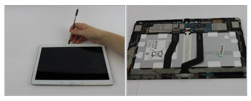
Using the <u>nylon spudger</u> or <u>plastic opening tool</u> along the edges of the screen, separate the back case off of the device.
