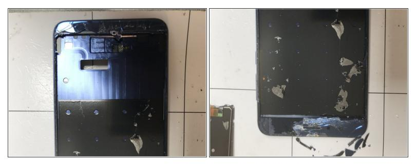
• Carefully remove the pieces of glass and the adhesive on the frame
