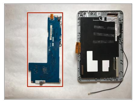
Gently, remove the motherboard by carefully lifting it.
