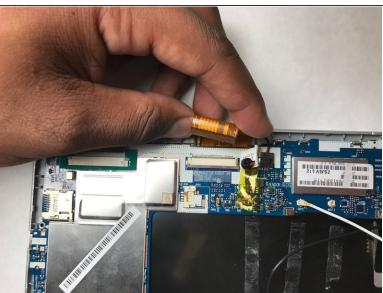
Next, unplug the orange strip from the motherboard by gently lifting it. The location of the orange strip is shown in the above picture, circled in red.
