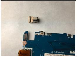
Remove the camera from the motherboard with the spudger.
