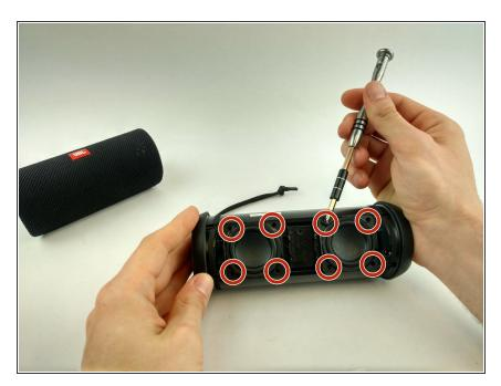
Remove the 8.9mm Phillips #00 screws on each corner of the driver to be replaced. There are four screws per driver. Be sure to set the screws somewhere safe to ensure they aren't lost.
