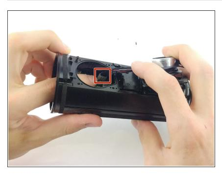
Remove the 3-pin connector from motherboard.
