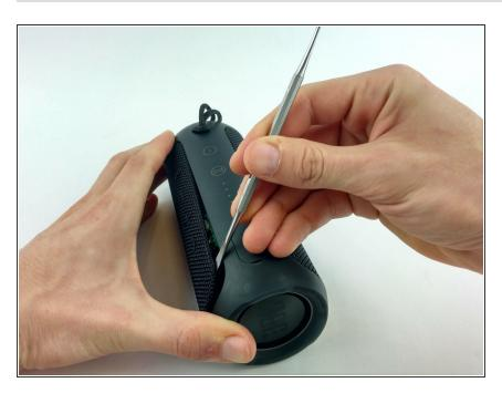
Remove plastic outer housing using hands or a standard spudger.
