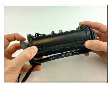
Using your hands, carefully remove outer housing and frame to expose the internal workings of the speaker.
