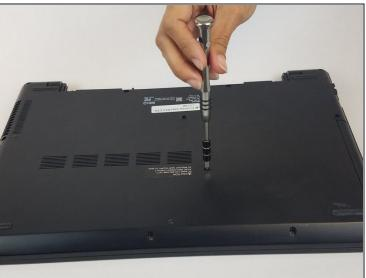
Unscrew the ten 6.5mm PH1 Phillips head screws that hold down the back cover.
