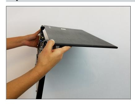
Open the laptop at a right angle to make the later removal much easier.
