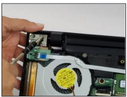
Unscrew the four PH1 Phillips head screws on the hinges.
