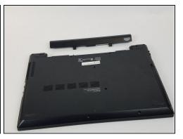
• Pull the battery out, keeping it flat and parallel to the laptop so that it slides out easily.
