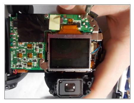
• Remove the 3 screws that attach the LCD screen to the circuit board.
