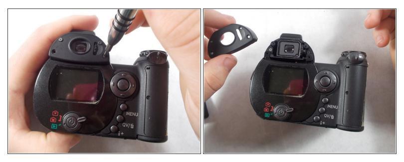
• Use a screwdriver to remove the four viewfinder cover screws.
