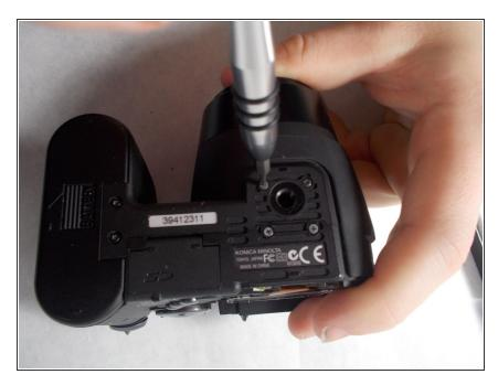
• Remove 6 screws on the bottom panel.
