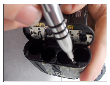
• Remove 1 screw inside the battery chamber.
