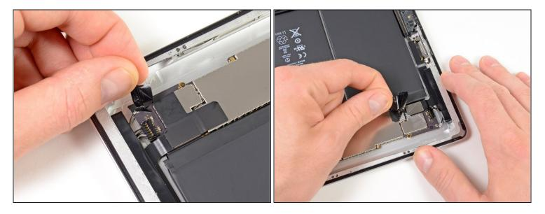
*i* If present, remove the pieces of electrical tape covering the Wi-Fi antenna, speaker cable, and dock connector cable.
