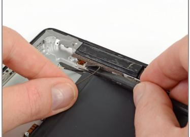
• Using the flat end of a spudger, release the adhesive tape holding the cellular data antenna cable to the aluminum frame.
