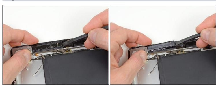
• Gently lift the cellular data antenna out of its housing in the iPad, using a spudger if necessary.
