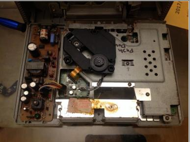
Pick up on the top case after you have flipped it over. This will have a little resistance but this should not break anything if you have all of the five screws out of the under case.
