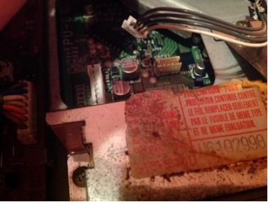
• Then undo the power cable and the eye Cable these should just lift right off.
