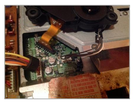
Then undo the piece holding in the ribbon cable. When you do this grab the side of the black piece holding it in place and pick it up slowly
