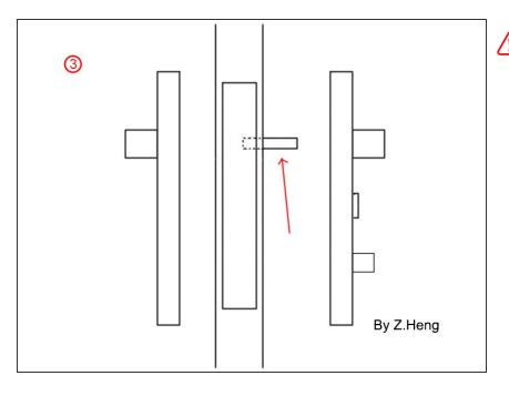
Pay attention to the installation direction of this square shaft. Do not knock it off when removing the handle.
