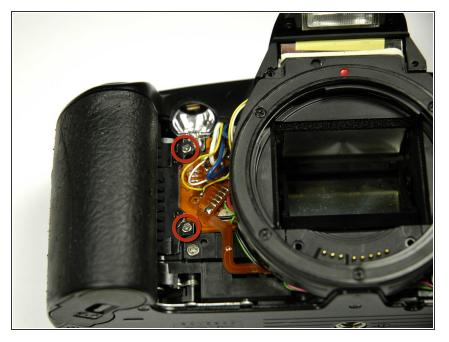
Using a 00 Phillips screw driver, unscrew the two 4.9 mm Phillips screws. on the inside of the camera.
