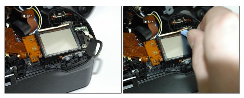
• Pry off the small metal brace holding the LCD screen. (Push forward and slide toward the center)
