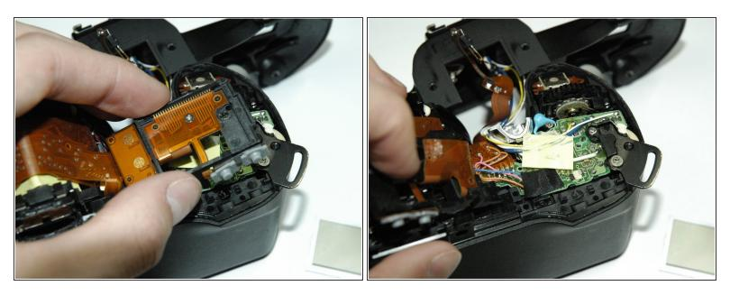
• Lift the LCD mount to reveal the logic board.
