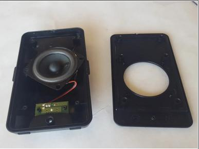
Once all seven 5mm screws are taken off use the metal spudger again to pry off the plastic casing from the speaker.
