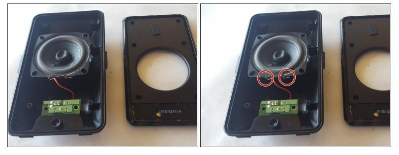
Follow <u>How To Solder and Desolder Connections</u> to desolder the speaker cone from the circuit board. To reassemble your device, follow these instructions in reverse order.
