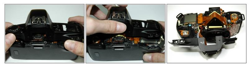
• Remove the top panel by lifting it from the back, pushing it forward over the camera and letting it rotate down in front of the camera.
