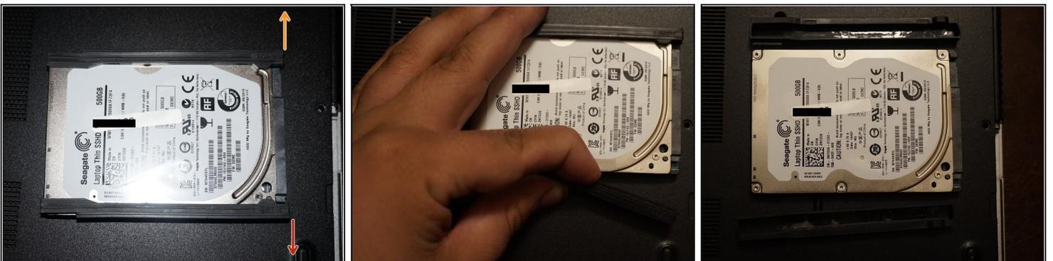
ⓘ The bumpers are held on with double sided tape. This does not have to be replaced.
