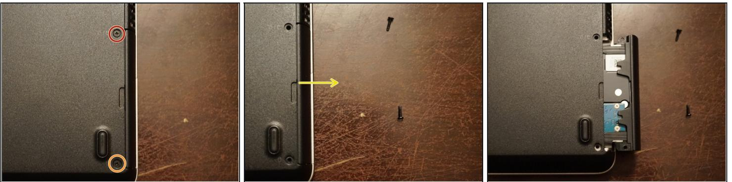
**⚠ The screw marked in orange is directly screwed into the chassis. *This point WILL break if overtightened.***
