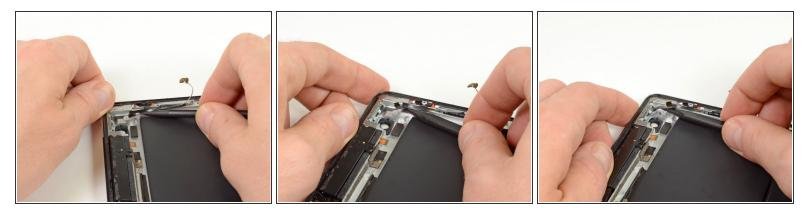
• Continue sliding the tip of the spudger toward the top of the iPad, releasing the adhesive.
