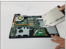
• Slide the disk drive to the right and gently lift up the disk out the laptop.
