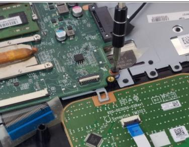
• Unscrew the seven PH1 Phillips head 3.0 mm long screws that hold the motherboard in place.
