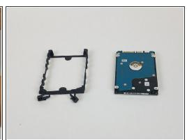
Peel off the rubber hard drive mount.
