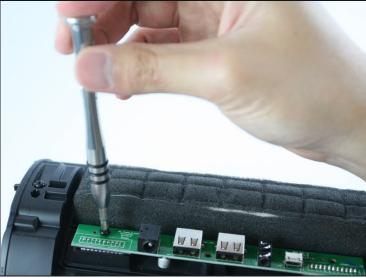
Unscrew the three 11.88mm Phillips head screws highlighted in the picture.
