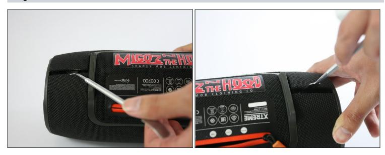
• Use the metal spudger to gently pry and lift the edge of the seam. The cover is held in place with plastic snaps that will make a popping noise when disengaged. !!Start with the back half, this will expose TWO Screws that need to be removed before lifting the front half.
