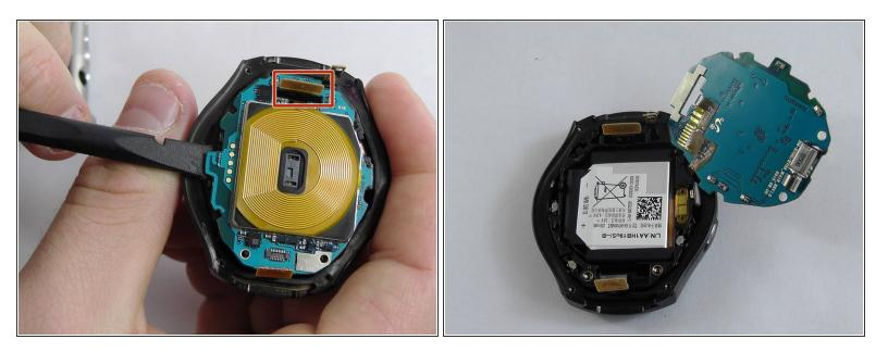
• Using the flat end of a spudger, pry up the motherboard.
