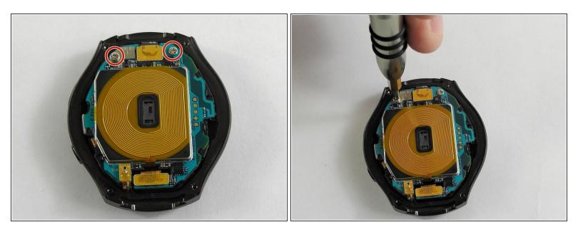
• Using a Philips head #00 screwdriver, remove the two 3.6 millimeter screws.
