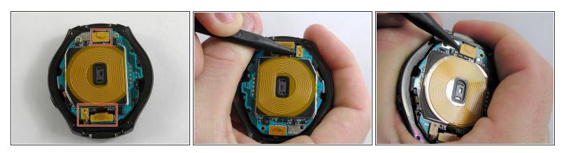
Using a spudger, pry up the three cables.
