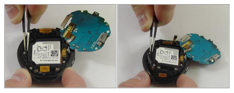
Using tweezers, lift the battery casing.
