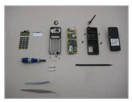
From left to right, top to bottom: Speaker, antenna, LCD screen, keypad, keypad support skeleton, front casing, circuit board, back casing, battery, screwdriver handle, paperclip, Torx T6 bit, SP2.6 U-bit, plastic pry bar, and two sets of tweezers.
