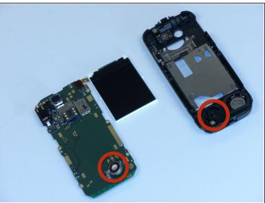
Using the plastic opening tool, gently pry off the motherboard from the plastic shell.
