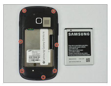
Find the positions of the seven screws on the back of the device. Use the Phillips #00 screwdriver to remove these 5.0mm screws.
