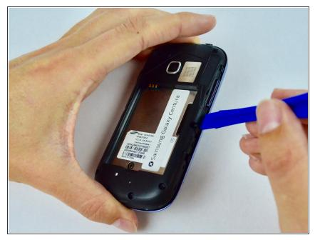
Gently insert the plastic opening tool into the notch on the side of the device. Apply a firm prying motion to pop open and remove the plastic casing.
