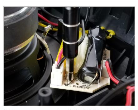
Remove the two 11 mm Philips #1 screws holding the filter to move it out of the way.
