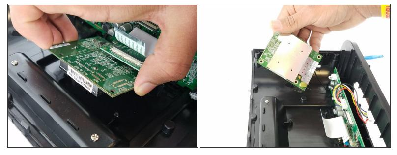
Lift the circuit board to expose the wifi antenna wire.
