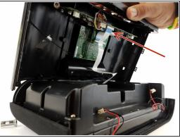
Separate the mesh frame and plastic frame by placing the spudger in between them.
