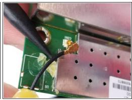
Pry the glue and unclip the wifi antenna plug from the circuit board.
