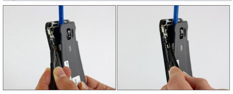
• Insert the tweezers under the contact points to undo the connection.
