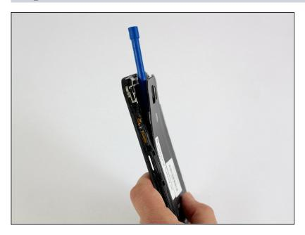
• Leave the plastic tool inside in order to access the power button connection.
