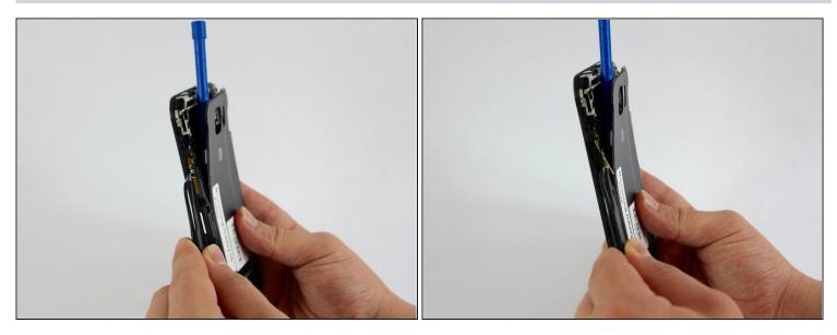
• Use the <u>tweezers</u> to pry up the power button ribbon cable until the only thing attached to the frame are the contacts.
