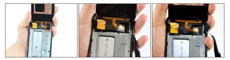
• Once the glass is off, you will see a small clip covering the screen connection to the motherboard at the top of the phone. Use <u>tweezers</u> to grab the clip by the crease on its side and pull it out.
