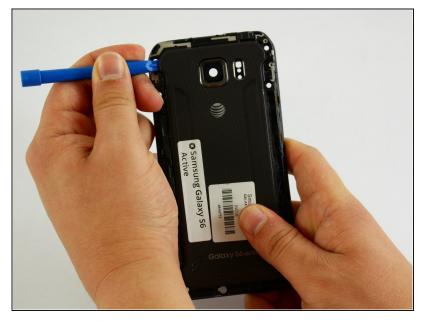
• Insert a plastic tool between the frame of the phone and the back cover at the top left corner.
