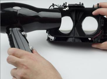
• Using a hairdryer (or heatlamp), warm the area around the lenses. This will help loosen them for removal.
