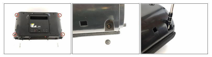
Remove the four 11 mm Philips #1 screws from beneath the rubber grommet that was removed from the previous step in all four corners.
