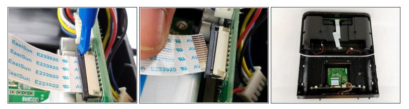
• Remove the ribbon cable by pulling the black clip towards the cable, then gently pull the ribbon cable to fully separate the mesh frame and plastic frame.
