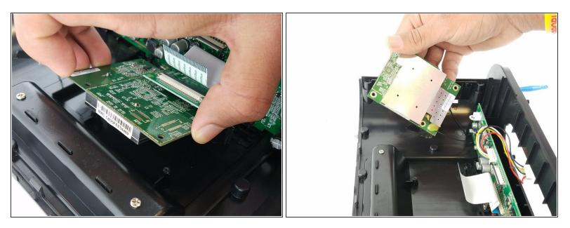
• Lift the circuit board to expose the wifi antenna wire.
