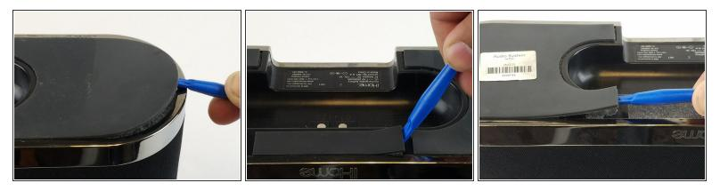
Remove the rubber from the bottom of the speaker, use a medium blue plastic spudger to gently work its way under the rubber and slowly peel off for each of the three feet. The order does not matter.
