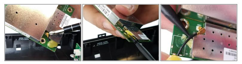
• Pry the glue and unclip the wifi antenna plug from the circuit board.
