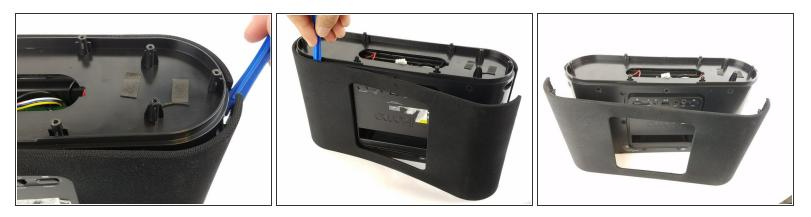
• Pry off the mesh frame from the back side of the speaker with a plastic spudger until you hear a click noise when the clip is removed.
