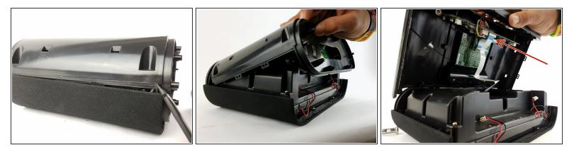
• Separate the mesh frame and plastic frame by placing the spudger in between them.
