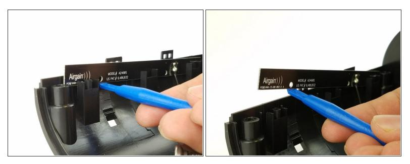
• Remove the wifi antenna from the side of the speaker by sliding it upward with a plastic spudger.
