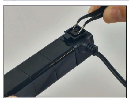
Using <u>tweezers</u>, remove the cap holding the cable grommet in place.
