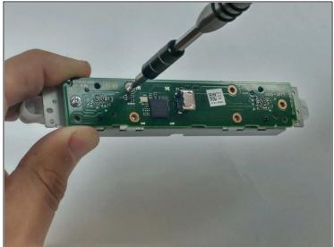
• Using the PH0 sized screwdriver, remove the six 4.2mm Phillips #0 screws securing the motherboard to the metal frame.
