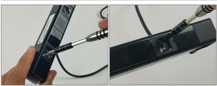
• Using the PH0 sized screwdriver, remove two 3.2mm Phillips #0 screws, located under the coverplates.
