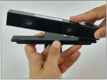
Separate the camera from the camera stand to gain access to the bottom of the camera.
