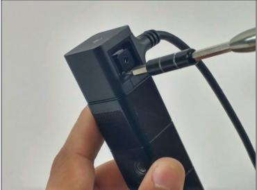
• Using a PH000 sized screwdriver, remove the two 6.5mm Phillips #000 screws located under the stand connection point, where the cable enters the case.
