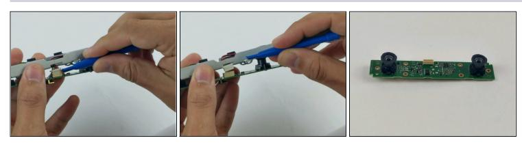
Using a plastic opening tool, disconnect the microphone array connector from the motherboard.
